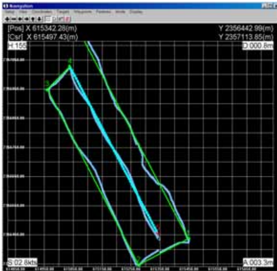
Figure 11. Planned track lines in green, and Dead-reckoned (DR) navigation for test survey in blue.
