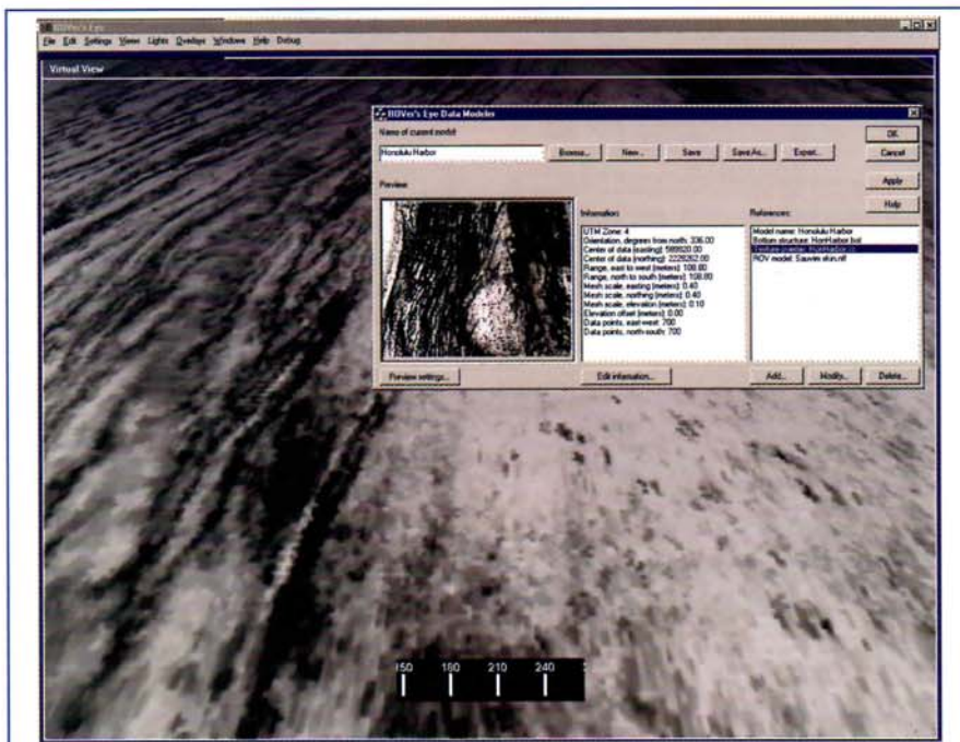
ROVER's Eye view of the bottom of Honolulu Harbor, with TargetView mode on, providing automatic notification of proximity of previously marked targets.
