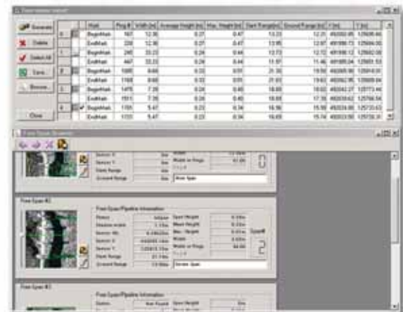
Free-span report and browse windows allow the user to check span areas and save project data to Excel spreadsheet for archiving and project management.
