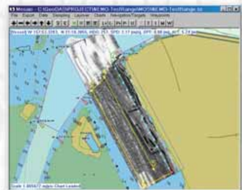
The RTM option displays a real-time evolving mosaic with vector shoreline data, with target data superimposed.
